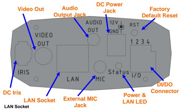
The LAN socket is a RJ-45 connector for connections to 10Base-T Ethernet or 100Base-TX Fast Ethernet cabling. This Ethernet port built N-Way protocol can detect or negotiate the transmission speed of the network automatically. Please use Category 5 "straight through" cable to connect the Network Camera to a 100Mbps Fast Ethernet network switch or hub. **Note** that, in case you need to connect the device to PC or notebook directly, you should use "cross-over" cable instead.
